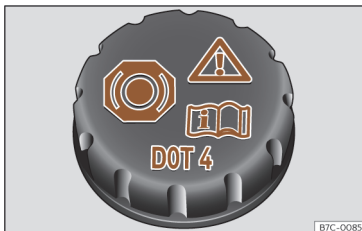
Fig. 211 Engine compartment: brake fluid reservoir cap.
