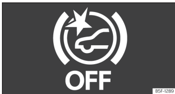
Fig. 137 On the screen of the instrument panel Front Assist switched off message.
