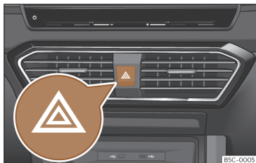
Fig. 49 Dashboard: switch for hazard warning lights.
