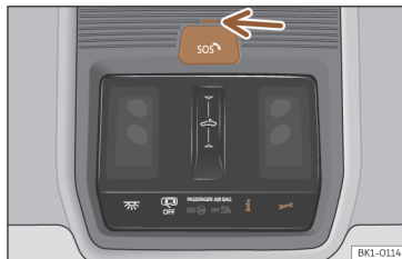
Fig. 50 On the roof console: controls for voice services.
