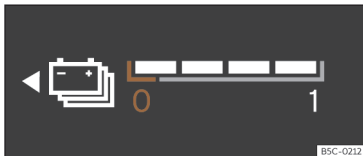
Fig. 5 Digital instrument cluster: battery level indicator.
