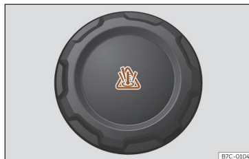
Fig. 210 Front compartment: coolant expansion tank cap.
