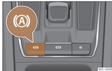
Fig. 147 In the lower part of the centre console: Auto Hold function button.
