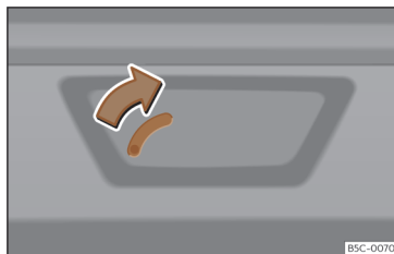
Fig. 80 Luggage compartment: manual release.
