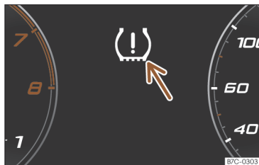
Fig. 229 Instrument panel: warning of loss of tyre pressure.
