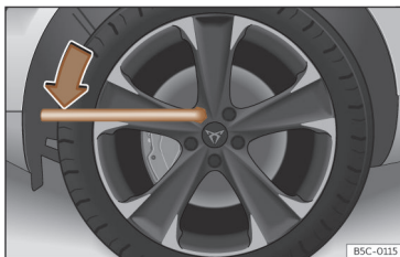
Fig. 226 Tyre change: slacken the wheel bolts.
