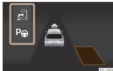
Fig. 132 On the instrument panel display: display of the assisted parking system with decreased visibility.
