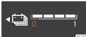
Fig. 5 Digital instrument cluster: battery level indicator.
