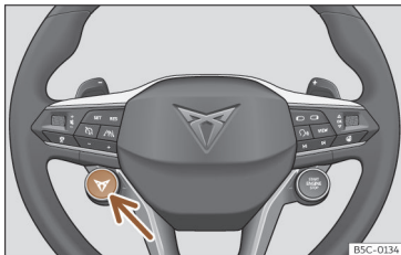
Fig. 117 Multifunction steering wheel: button to change the driving profile.
