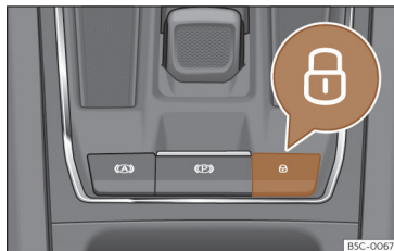
Fig. 71 On the centre console: central locking switch
