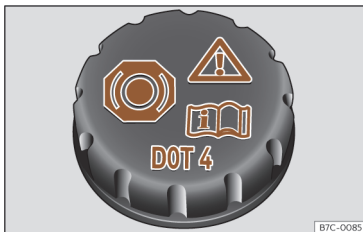
Fig. 219 Front compartment: brake fluid reservoir cap.
