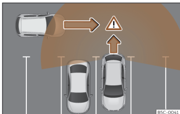
Fig. 155 Diagram of the parking assistant: detected area around the vehicle that is driving off.
