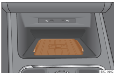
Fig. 170 Centre console: slot for mobile phone connection.
