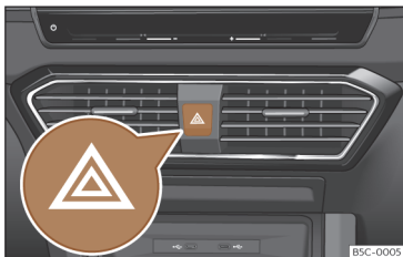
Fig. 49 Dashboard: switch for hazard warning lights.
