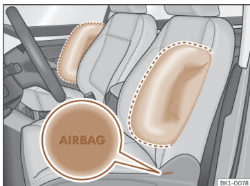
Fig. 33 Driver's seat and passenger seat side airbags.
