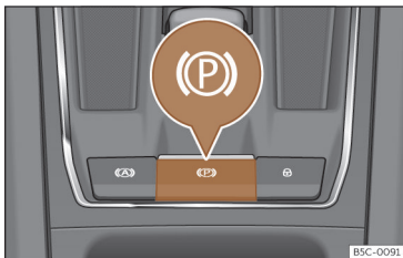
Fig. 145 Centre console, lower part: electronic parking brake button.
