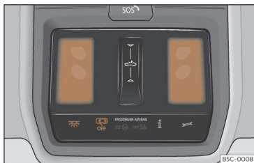
Fig. 101 Detail of headliner: front interior lighting.
