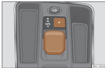
Fig. 115 On the centre console: selector lever.
