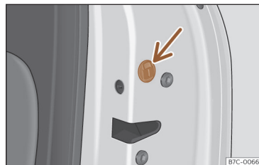
Fig. 73 Locking the door manually.
