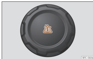
Fig. 218 Front compartment: coolant expansion tank cap.
