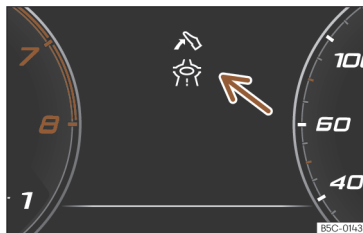
Fig. 10 Eco-efficient driving assistance indication (schematic representation).
