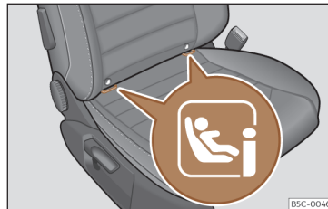
Fig. 42 Front passenger seat: location of the i-Size fastening rings.
