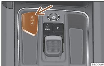
Fig. 64 Centre console: vehicle key housing.
